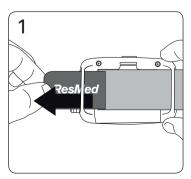
Thread one end of the belt through the slots on the back of the device. Check that the device is positioned as shown. Follow these steps if you are using the effort sensor:
