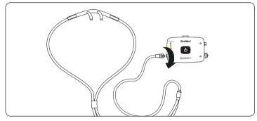
Unscrew and remove the protective cap and insert the connector end of the nasal cannula into the nasal cannula connector on the device. Turn clockwise until the connector is secure.
