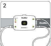
Check that lights next to the accessories you are using are green. If any of these lights are red and blinking, the accessories are not attached correctly.
