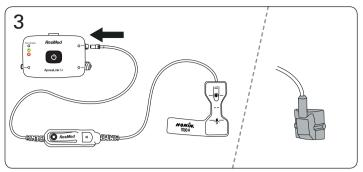
3. Attach the oximeter to the oximeter connector on the device by pushing it on.
