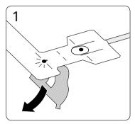
1. Remove the backing from the sensor.
