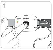
Press and hold the power button in the centre of the device for about three seconds or until the light turns on.
