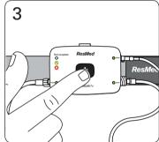
Press and hold the power button for about three seconds to turn off the device.
