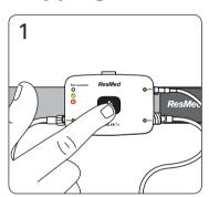
**1.** Press the power button for about three seconds.
