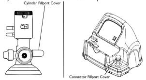
5. When the cylinder fillport is disconnected from the connector fillport, release the outer ring (sleeve) of the connector fillport and use two hands to remove the cylinder from the compressor cradle.
