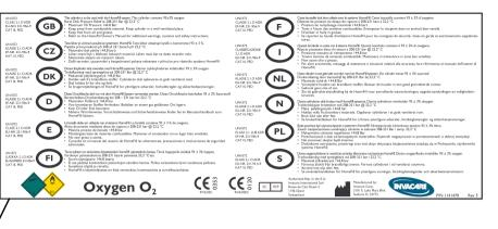
This cylinder is to be used with the HomeFill system. This cylinder contains 93±3% oxygen. Burst Disk Pressure Relief at 208-231 Bar @ 22.2°C. Keep cylinder in a well ventilated place Keep away from combustible material. Keep free from oil and grease. Refer to the HomeFill Owner's Manual for additional warnings, cautions and safety instructions.
