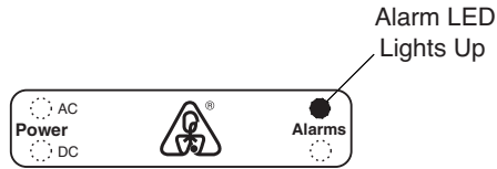
Figure 7-3 Alarm LED Lights Up
