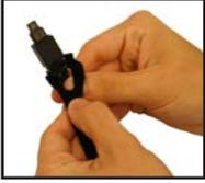
1. Wrap the end tabs of the retainer strap around the charging cord connector.
